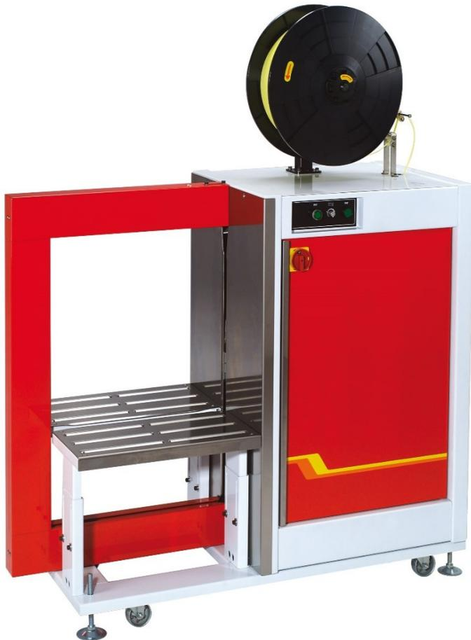
**Automatic strapping machine with arch for PP strapping.**
